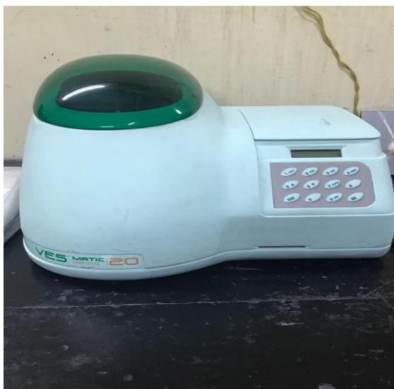
Figure 2: Automated Ves-Matic 20/20 Plus New For ESR Estimation
